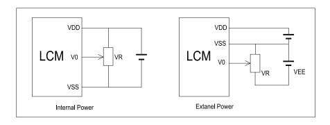
VDD~V0: LCD Driving voltage
