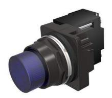
30mm BlackMax, Epoxy Coated Corrosion Resistant Complete Metal Unit Illuminated Indicator Light Transformer type, 600V AC LED Lamp, BA9s Plastic Lens, Blue UL Listed, CSA Certified NEMA 1,3,3R,4,4X,12,13 & Automotive Standards
