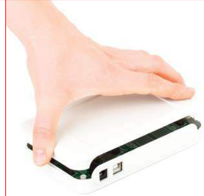
Figure 8-3: Place plastic casing cover and wind screws into outer screw holes to fix it with bottom plastics casing
