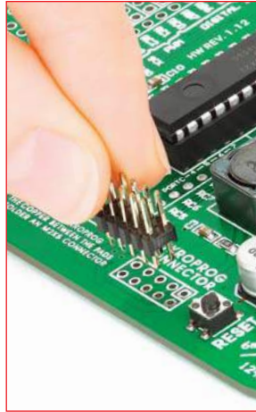
Figure 3-3: placing 2x5 male header
