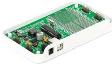
Figure 8-2: Wind screws into inner screw holes to fix the board with the bottom plastic casing
