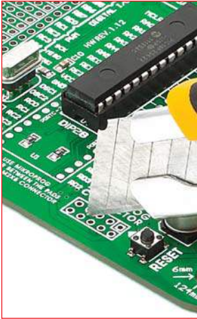
Figure 3-2: cutting copper between pads
