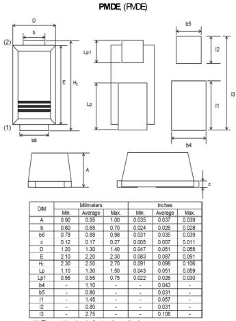
(1) The marking bar indicates the cathode.(2) The direction indicates the anode.
