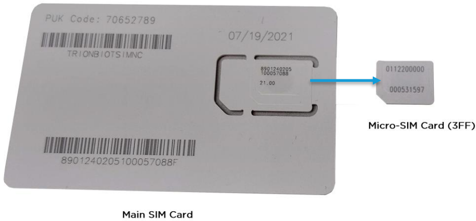
Figure 6: SIM Card Punch-Out
