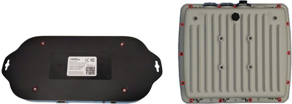
Figure 4: Gateway Screw Locations (Left: Standard; Right: IP67)
