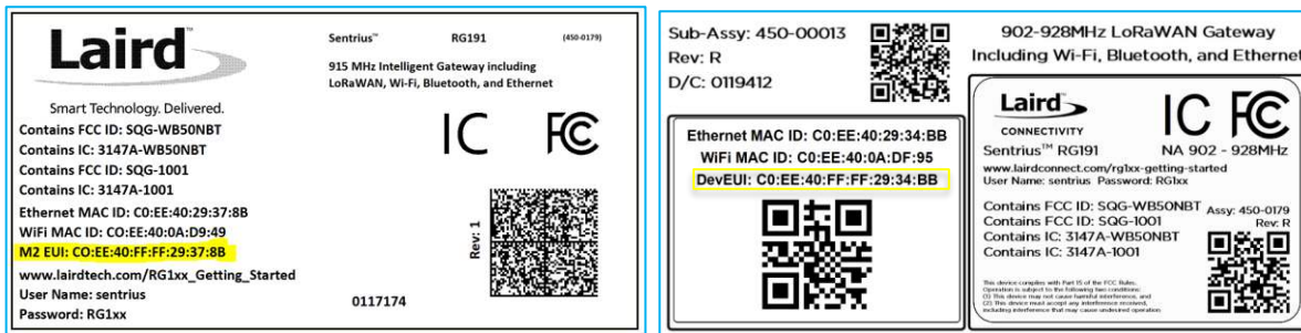
Figure 28: Gateway label (Standard GW – Left, AS923 & AU915 Region Supported/Latest Version – Right)
