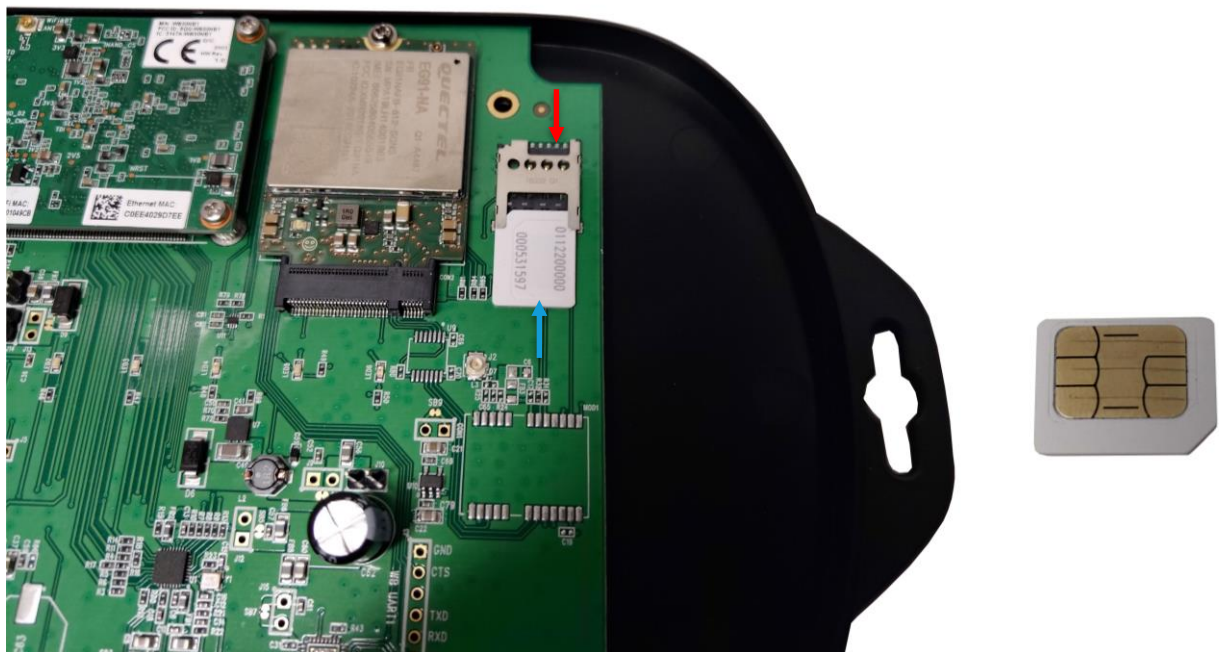
Figure 7: SIM Install (Right: Picture of SIM card contact side)
