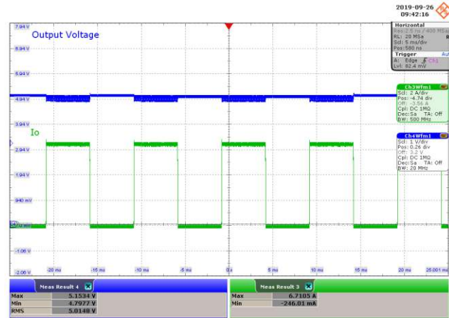
Figure 46 – Transient Response. 135 VAC, 5 V, 0 – 6.5 A Load Step. V_{MIN} : 4.797 V, V_{MAX} : 5.153 V. Upper: V_{OUT} , 1 V / div., 5 ms / div. Lower: I_{LOAD} , 2 A / div.
