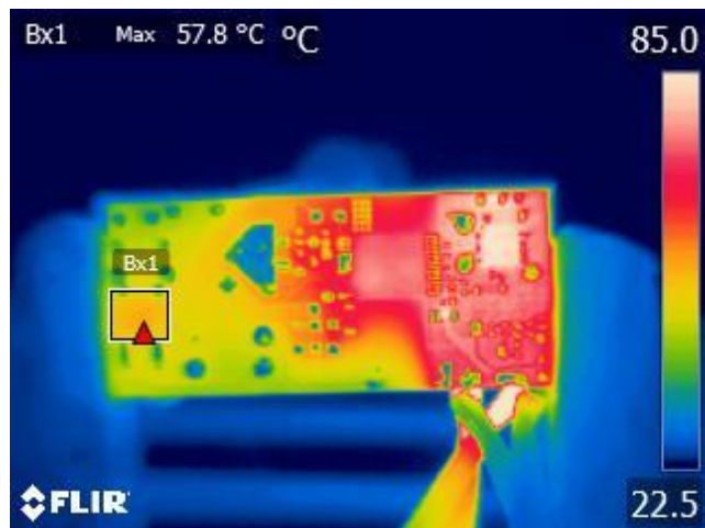
Figure 39 – Ambient = 22.5 °C. Bridge Diode, BR1 = 57.8 °C.
