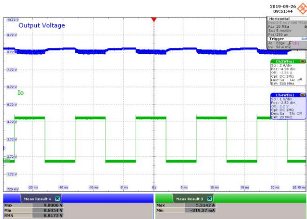
Figure 47 – Transient Response. 100 VAC, 9 V, 0 – 5 A Load Step. V_{MIN} : 8.605 V, V_{MAX} : 9.000 V. Upper: V_{OUT} , 1 V / div., 5 ms / div. Lower: I_{LOAD} , 2 A / div.
