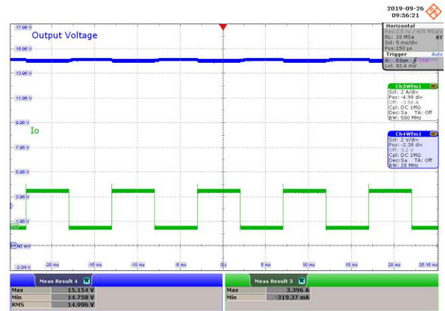
Figure 50 – Transient Response. 135 VAC, 15 V, 0 – 3 A Load Step. V_{MIN} : 14.758 V, V_{MAX} : 15.154 V. Upper: V_{OUT} , 2 V / div., 5 ms / div. Lower: I_{LOAD} , 2 A / div.
