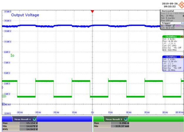
Figure 49 – Transient Response. 100 VAC, 15 V, 0 – 3 A Load Step. V_{MIN} : 14.679 V, V_{MAX} : 15.154 V. Upper: V_{OUT} , 2 V / div., 5 ms / div. Lower: I_{LOAD} , 2 A / div.
