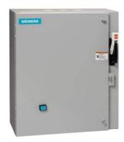
2-speed 3-phase motor starter Size 0 One winding consequent pole Constant or variable torque Solid-state overload relays Low SPD OLR range 0.75-3.4A High SPD OLR range 0.75-3.4A 110V 50HZ / 120V 60HZ coil Combination type 3Amp circuit breaker Enclosure NEMA type 1 Indoor general purpose use
