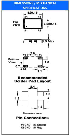
\*Dimensional drawing is for reference to critical specifications defined by size measurements.
