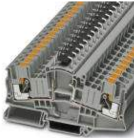
Component terminal block, Connection method: Push-in connection, Cross section: 0.5 mm 2 -10 mm 2 , AWG: 20 - 10, Width: 8.2 mm, Color: gray
