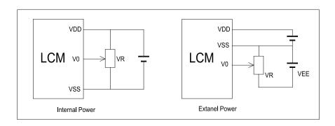
VDD~V0: LCD Driving voltage VR: 10k~20k
