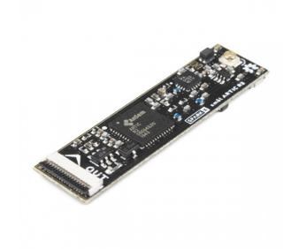
The smôl ARTIC R2 Peripheral Board is a complete satellite transceiver for the ARGOS satellite network.
