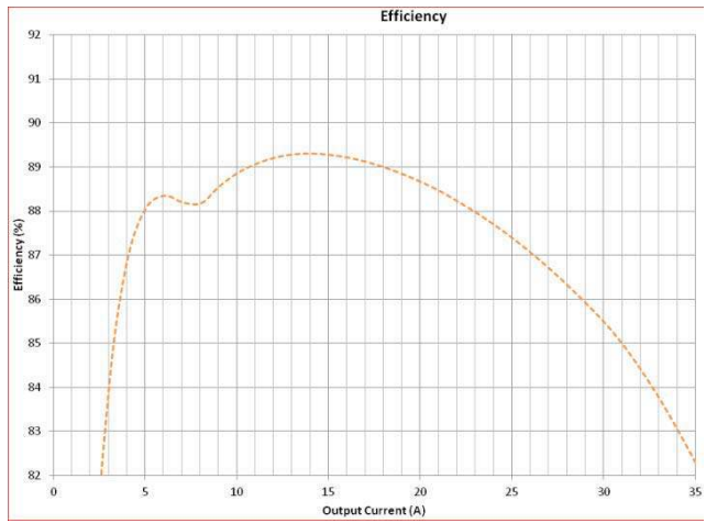
Figure 5. Efficiency – 19 V Input, 1.2 V Output, 500 kHz
