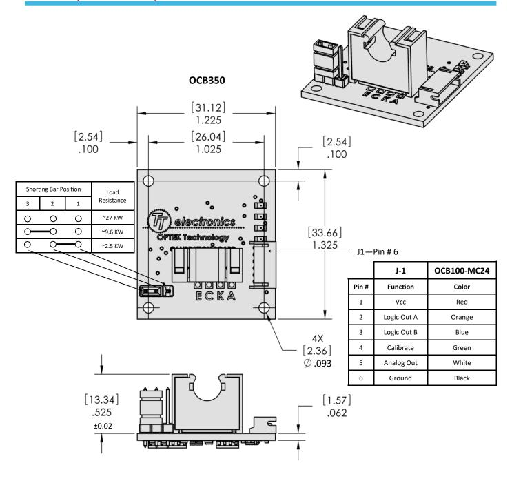
OPB350 / OCB350 Series (Calibration Circuit Available) Obsolete (OPB350C125Z)
