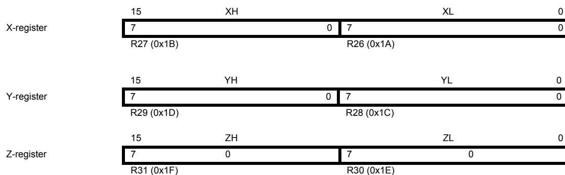
Figure 7-3. The X-, Y- and Z-registers.
