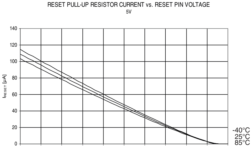
Figure 30-263. ATmega3250A: Reset Pull-up Resistor Current vs. Reset Pin Voltage ( V_{CC} = 5V )
