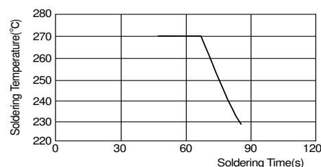
[Allowable Reflow Soldering Temperature and Time]
