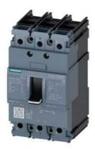
circuit breaker 3VA5 UL frame 125 breaking capacity class S 25kA @ 480 V 3-pole, line protection TM210, FTFM, In=25A overload protection Ir=25A fixed short-circuit protection Ii=12 x In nut keeper kit on both sides
