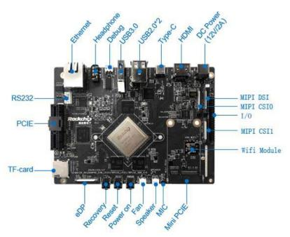
The TB-RK3399Pro development board has rich external interfaces, including 4 lanes PCIE and Mini PCIE, dual high-speed USB3.0 port Type-C + USB3.0 Type-A, dual MIPI CSI and dual ISP with pixel processing capability up to 1300W pixels, and HDMI2.1, DP1.2, MIPI-DSI and EDP; it also supports 8-channel digital microphone array input.
