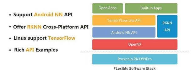
On the software side, TB-RK3399Pro is pre-installed Android and Linux system, support dual system boot and one-button OS switching. integrated rich AI application development components, providing friendly and concise application programming interface, seamless docking NPU to achieve AI computing hardware acceleration, support Various model inferences such as TensorFlow/TensorFlow lite/Caffe.
