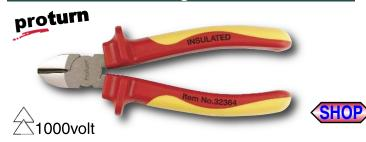
323 Proturn Insulated Diagonal Cutters. Insulation According to VDE 0682/part 201, DIN 7437, EN/IEC 60900, ASTM F-1505-01, NFPA70E, 1000 volt rated. Individually Tested. DIN ISO 5745 Pliers drop-forged from special tool steel, individually high frequency induction hardened, chrome and nickel plated, mirror polished. Proturn ergo soft grip handles for maximum comfort.
