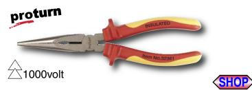
323 Proturn Insulated Long Nose Pliers. Insulation According to VDE 0682/part 201, DIN 7437, EN/IEC 60900, ASTM F-1505-01, NFPA70E, 1000 volt rated. Individually Tested. DIN ISO 5745 Pliers drop-forged from special tool steel, individually high frequency induction hardened, chrome and nickel plated, mirror polished. Proturn ergo soft grip handles for maximum comfort.
