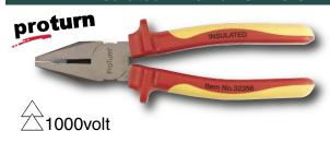
323 Proturn Insulated Lineman's Pliers. Insulation According to VDE 0682/part 201, DIN 7437, EN/IEC 60900, ASTM F-1505-01, NFPA70E, 1000 volt rated. Individually Tested. DIN ISO 5745 Pliers drop-forged from special tool steel, individually high frequency induction hardened, chrome and nickel plated, mirror polished. Proturn ergo soft grip handles for maximum comfort.
