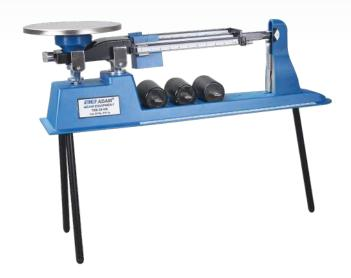
Created to withstand daily student use, Adam Equipment's patented TBB triple beam balance offers the best value for teaching mass measurement concepts. With rugged construction and security slot to prevent theft, the durable TBB is ideal for classroom environments. Other features include sturdy tripod legs for density measurement, weigh-below hook, magnetic damping for faster stability, notched and tiered graduated beams with center reading, and holders for storing extra weights.
