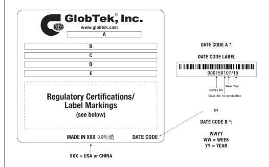
A=ICT / ITE / Medical Power Supply B=P/N: (料号) GTM91110P15015FSIM(R C=Model (型号) GTM91110P24015-F-S D=Input (输入)100-240V~, 50-60 Hz, 4.0A E=Output (输出)15.0 V == 10.0 A, 150.00W
