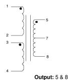
Input (115V): Input 1 & 2 Connect 1&3, 2&4 Input (230V): Input 1 & 4
