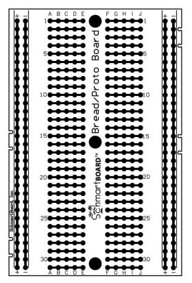
400 Tie Point Schmartboard Bread/Proto Board Bundled with a 400 Point Breadboard
