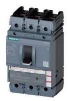
circuit breaker 3VA5 UL frame 250 breaking capacity class M 35kA @ 480 V 3-pole, line protection TM210, FTFM, In=90A overload protection Ir=90A fixed short-circuit protection Ii=10 x In UL489 SB (naval), 50 deg. cel. nut keeper kit on both sides
