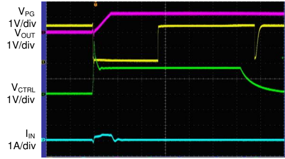
V CTRL Start up and Shut down Waveform (V CTRL =0 to 5V, V EN =5V, V IN =2.2V, No Load)
