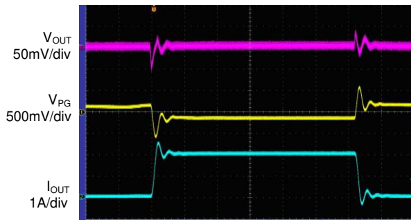
Load Transient (V CTRL =V EN =5V, V IN =2.2V, I OUT =0 to 2A)
