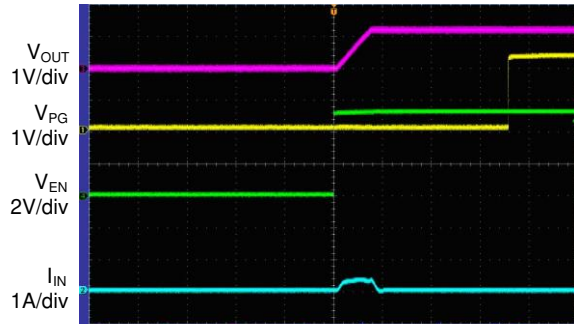
V EN Start up Waveform (V CTRL =5V, V EN =0 to 5V, V IN =2.2V, No Load)
