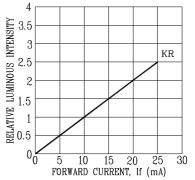
Fig3. Relative Luminous Intensity vs. DC Forward Current
