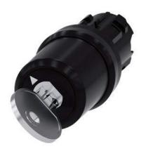
Key-operated switch BKS, 22 mm, round, plastic, lock number S1, with 2 keys, 2 switch positions O-I, latching, actuating angle  $90^\circ,\,10:30h/13:30h,$  key removal I, with laser labeling, inscription or symbol Customer-specific selection with SIRIUS ACT configurator (CIN)
