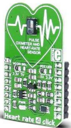
**Heart rate 4 click** carries the MAX30101 high-sensitivity pulse oximeter and heart-rate sensor from Maxim Integrated. The click is designed to run on either 3.3V or 5V power supply. It communicates with the target MCU over I2C interface, with additional functionality provided by INT pin on the mikroBUS™ line.
