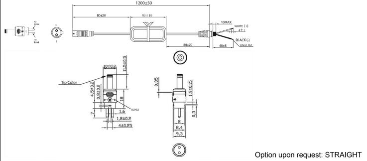
Female Barrels are available for special order in any length between 9mm-14mm
