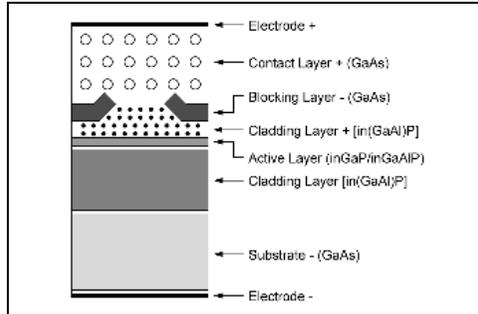
Figure 20. Index-Guided Visible Laser Diode (VLD), Schematic Structure
