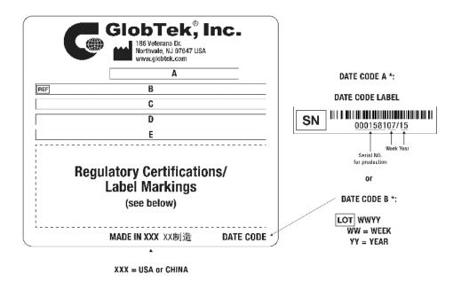
A=ICT / ITE / Medical Power Supply B=P/N: (料号) TR9KR4000T00-IM(R6B) C=Model (型号) GTM961200P12030-T2 D=Input (输入)100-240V~, 50-60 Hz, 1.5 A
