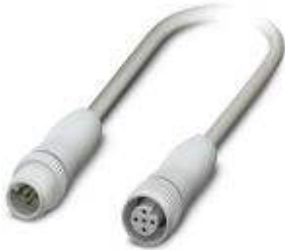
Sensor/Actuator cable, 5-position, PP-EPDM halogen-free, Gray RAL 7035, Plug straight M12, A-coded, on Socket straight M12, A-coded, Cable length: 3 m, Hygienic design, with plastic knurl
