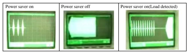
Note: The minimum power of a load to take inverter out of sleep mode (Power Saver On) is 50 Watts.
