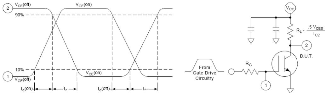
Figure 16, Resistive Switching Time Test Circuit and Waveforms
