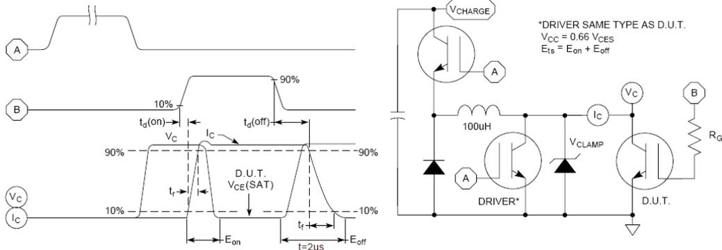
Figure 15, Switching Loss Test Circuit and Waveforms
