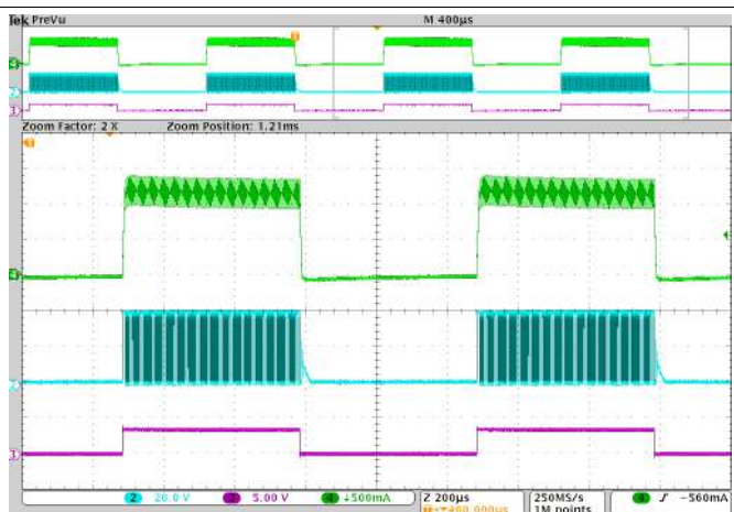
CH4: Inductor Current CH3: PWMx Pin CH2: SWNx Figure 27. PWM Dimming, Two Periods
