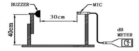
MIC: S.P.L meter TES1351B or equivalent
