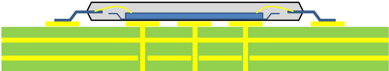
Figure10.2-1: Example thermal via holes on PCB.
