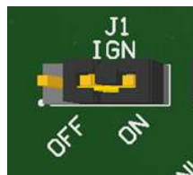
Figure 17. Ignition Jumper Configuration Default: ON (Device powers up when power is applied)
