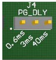
Figure 20. Power-Good Delay Selection Jumper Configuration Default: Jumper Not Installed, 3-ms Delay
