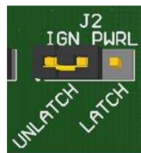
Figure 18. Power-Latch Jumper Configuration Default: LATCH
