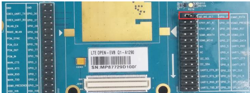
Figure 30: eMMC Function GPIO Configuration
