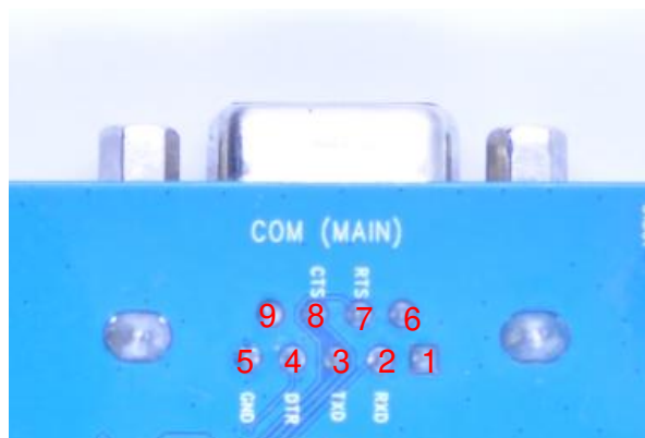
Figure 33: Pin Assignment of J0502
