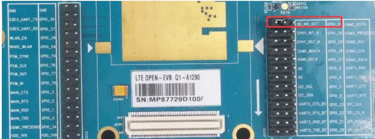
Figure 29: SD Card Function GPIO Configuration
