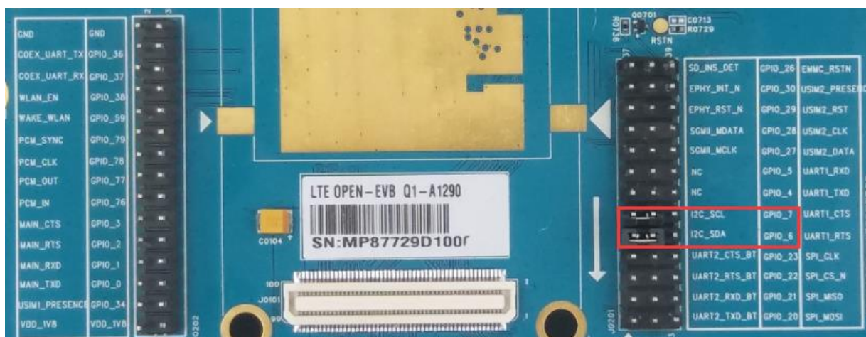
Figure 39: EEPROM Function GPIO Configuration
