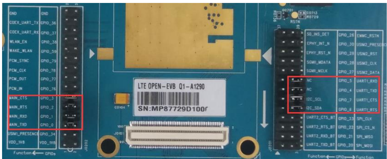
Figure 35: COM (MAIN) & COM (UART1) Function GPIO Configuration
