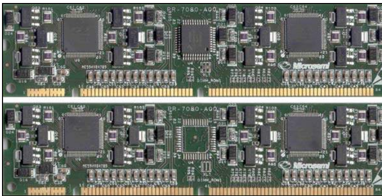
Figure 1: PoE PD67124 DIMM
