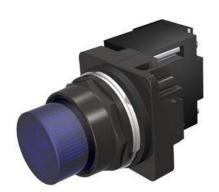
30mm BlackMax, Epoxy Coated Corrosion Resistant Complete Metal Unit Illuminated Indicator Light Transformer type, 240V AC LED Lamp, BA9s Plastic Lens, Blue UL Listed, CSA Certified NEMA 1,3,3R,4,4X,12,13 & Automotive Standards
