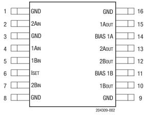
Figure 2. ACA2431 Pinout (Top View)
