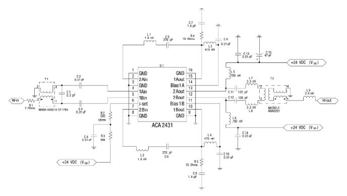
Figure 3. ACA2431 Evaluation Board Schematic
