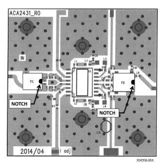
Figure 4. ACA2431 Evaluation Board Assembly
