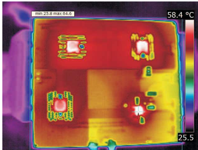
Figure 6. TL4242EVM-543 Top Infrared at V_{in} = 12\text{ V} , I_{LED} = 357\text{ mA} (Viewed From Top)
