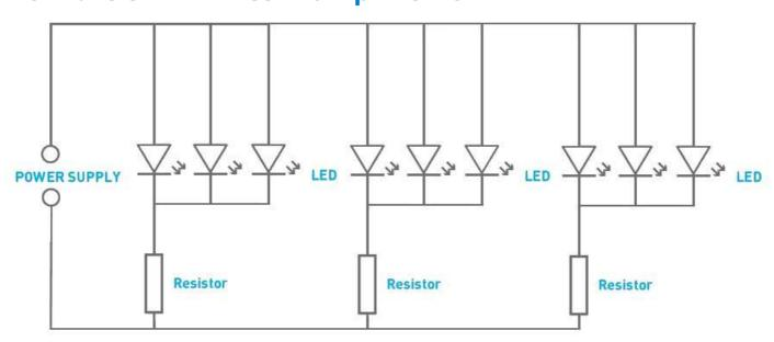
The circuit diagram for the 5V LED Desk Lamp is shown above. It is a very simple circuit. The board contains nine LEDs, these are grouped in to threes, with each group of three sharing a current limit resistor.
