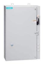
Non-reversing motor starter, Size 3, Three phase full voltage, Solid-state overload relay, OLR amp range 25-100A, 240V 50Hz / 277V 60Hz coil, Combination type, 100A fusible disconnect, 100A/600V fuse clip, Encl NEMA type 4X 304 S-Steel, Water/dust tight noncorrosive, Standard width enclosure
