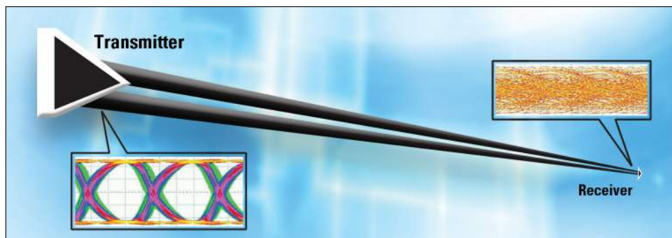
Figure 1: Typical Signal Deterioration Over Long Channels
