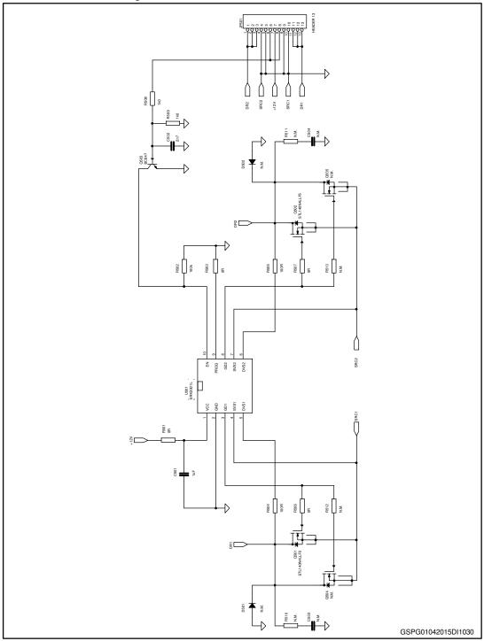
Figure 1: STEVAL-ISA169V1 circuit schematic
