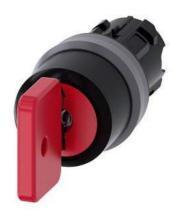
Key-operated switch O.M.R, 22 mm, round, plastic with metal front ring, lock number 73037, red, with 2 keys, 3 switch positions I>O<II, momentary contact type, actuating angle 2x45°, 10:30h/12h/13:30h, key removal O, with laser labeling, inscription or symbol Customer-specific selection with SIRIUS ACT configurator (CIN)
