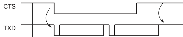
Figure 48-28: Transmitter Behavior when Operating with Hardware Handshaking
