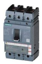
circuit breaker 3VA5 UL frame 250 breaking capacity class C 100kA @ 480 V 3-pole, line protection TM230, FTAM, In=80A overload protection Ir=80A fixed short-circuit protection li=5...10 x In nut keeper kit on both sides
