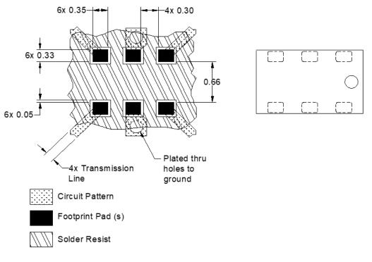
Dimensions are in Millimeters Mounting Footprint
